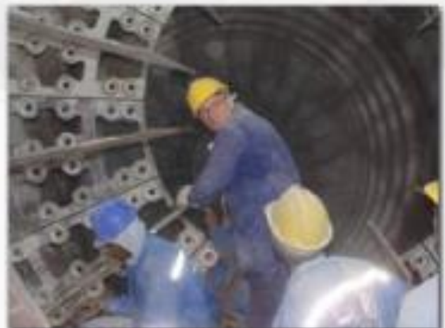
Replacement of Diaphragm - TOURAH Plant II Line 9
