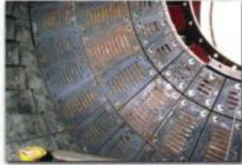
Cement Mill Diaphragm Liner
